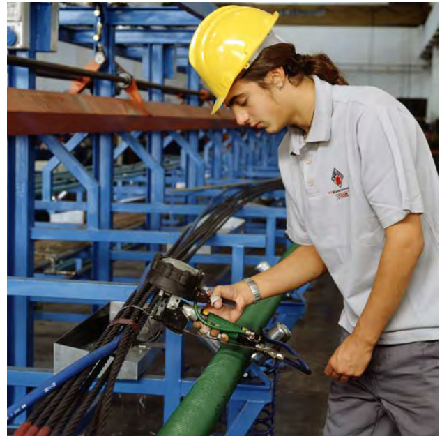
Spacer strapping on the bulb
