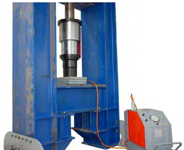
Pressure calibration on a TTM hydraulic pump
