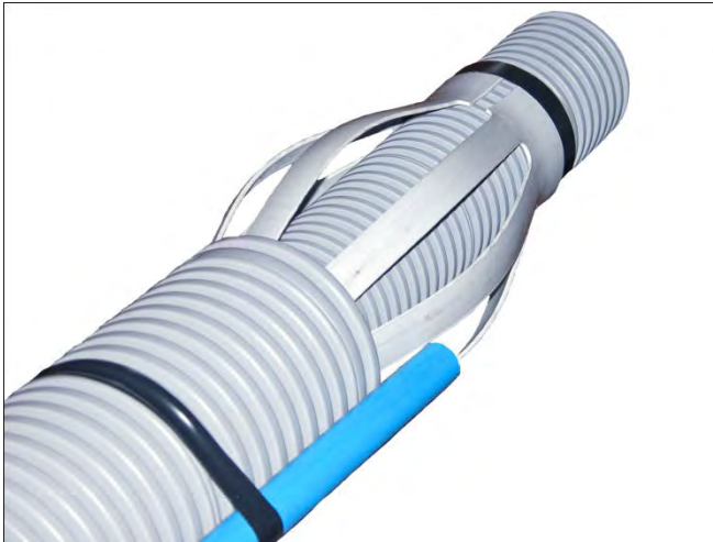
Anchor encapsulated in a double protection with external grout within 16x20 mm tube.
