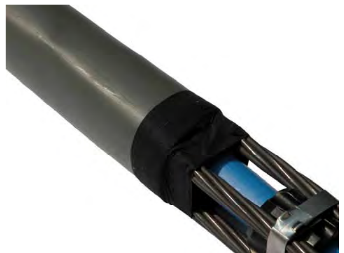
Buffer for TPR 01 temporary ground anchors and protection of the free length with a smooth sheath
