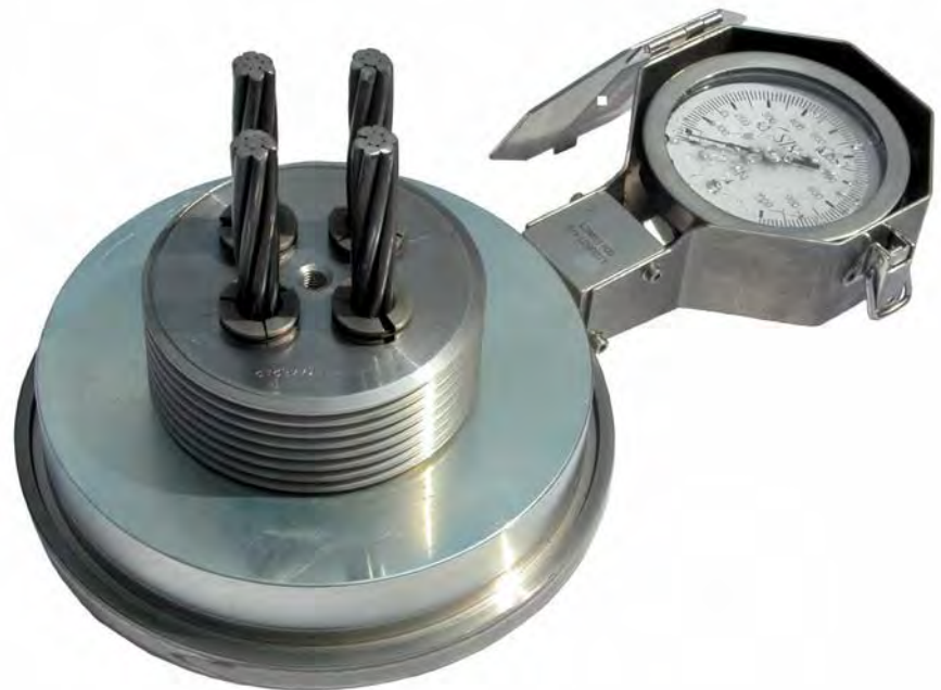
Load cell with 4 TTM-F15 plate
