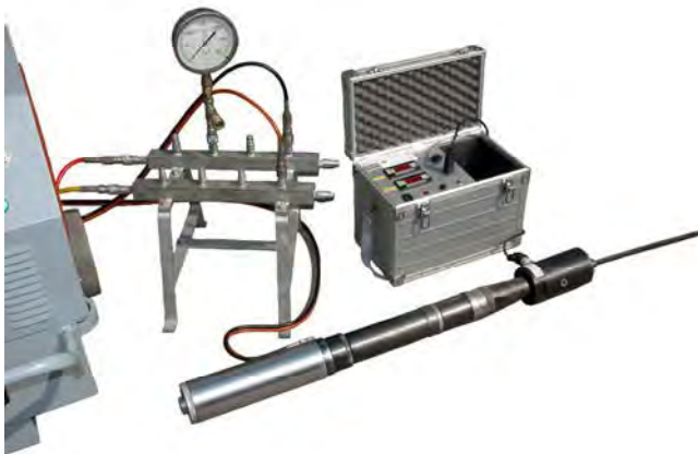
Calibration of TTM jack and related pump.
