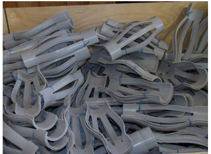
DD-ED spacers supplied in two halves
