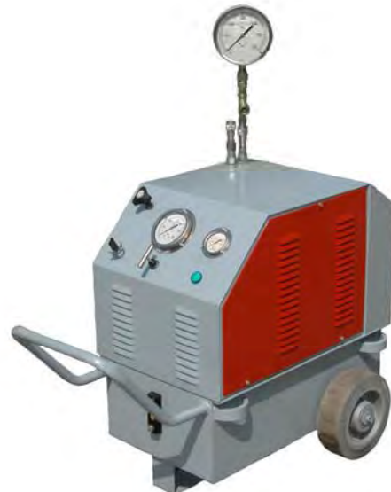
Pressure calibration on a TTM hydraulic pump
