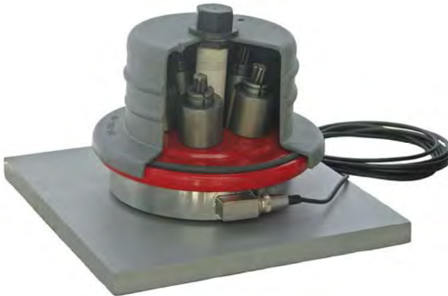
DE1000KN cell on TTR-100 anchorage
