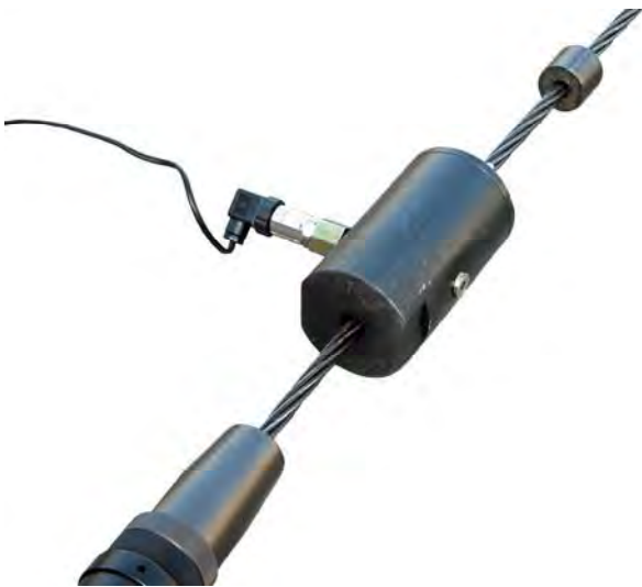
S300KN hydraulic transducer
