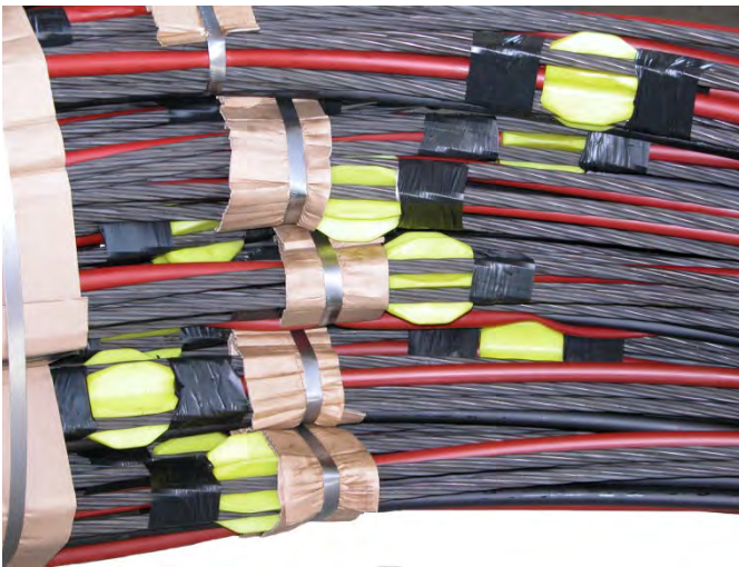
DD CT centralizer mounted on rolled up anchors
