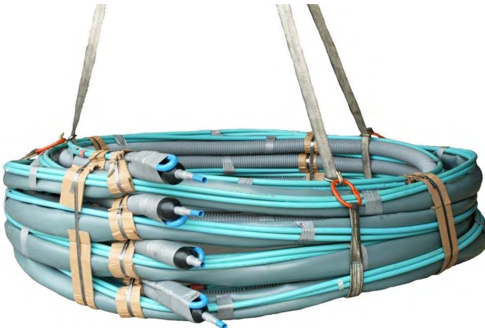
TPE-08B anchor provided with corrugated sheath on the foundation and smooth sheath on the free length.
