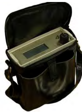
TT2000 reading device for DE cells
