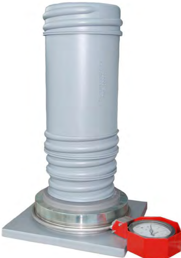
DI load cell with distribution plate and long cap
