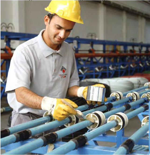
RRM valves gluing on a 27x34 mm valvate tube
