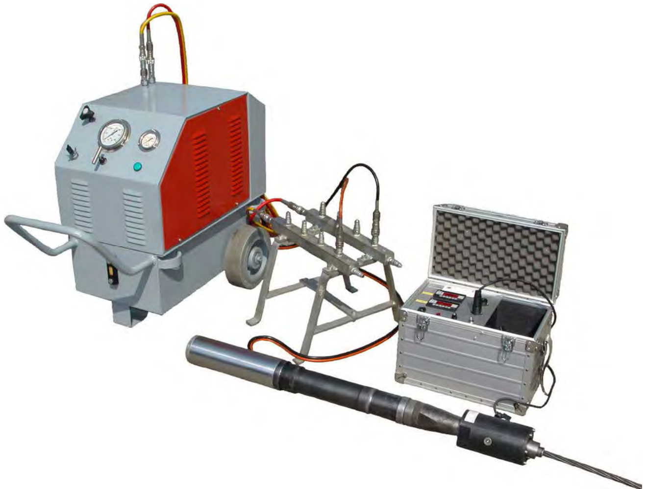
Equipment being calibrated with S1000 gauge box and S300KN hydraulic transducer
